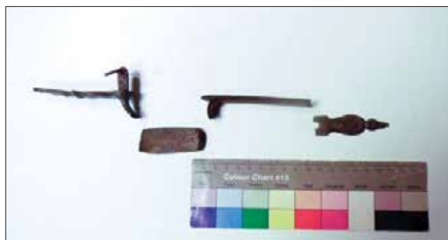
Obr. 4. Granátometná puška Z 11, poškozený lučík pušky, stav po požáru. Foto Petr Vaníček / Grenade launcher Z 11, damaged trigger guard, condition after the fire. Photo Petr Vaníček
