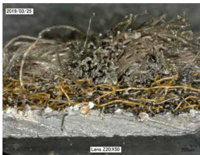
Obr. 8. Koberec pod mikroskopem – podkladová vrstva a vlákna / Carpet under the microscope – foundation layer and fibres
