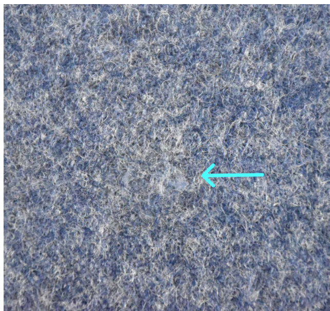
Obr. 10 Modré sukno, detail perforace po konsolidaci (lícová strana). Foto © TMB / Blue cloth, detail of perforation after consolidation (face side). Photo © TMB
